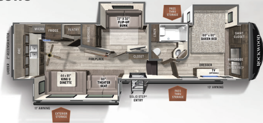
2887MB BUNKHOUSE ULTRA LITE U/VW: 10229 HITCH: 1620 AXLE: 8550 CCC: 1791 LENGTH: 36' 6" WIDTH: 8' HEIGHT: 13' 2" FRESH: 54 gal GRAY: 90 gal BLACK: 50 gal
