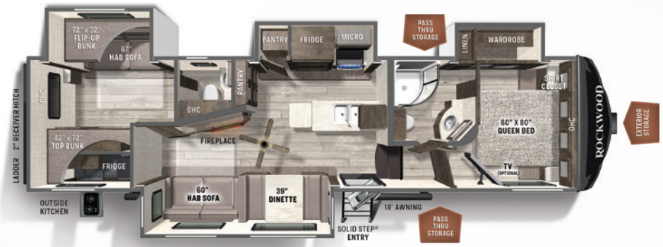
2892RB BUNKHOUSE ULTRA LITE U/VW: 10018 HITCH: 1602 AXLE: 8357 CCC: 1584 LENGTH: 36' 6" WIDTH: 8' HEIGHT: 13' 4" FRESH: 54 gal GRAY: 90 gal BLACK: 90 gal
