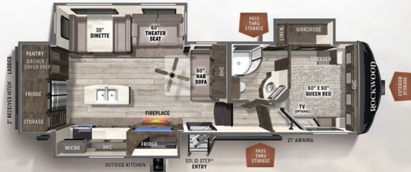
2882S REAR KITCHEN ULTRA LITE U/VW: 9620 HITCH: 1496 AXLE: 8065 CCC: 1876 LENGTH: 33' WIDTH: 8' HEIGHT: 13' 2" FRESH: 54 gal GRAY: 70 gal BLACK: 40 gal
