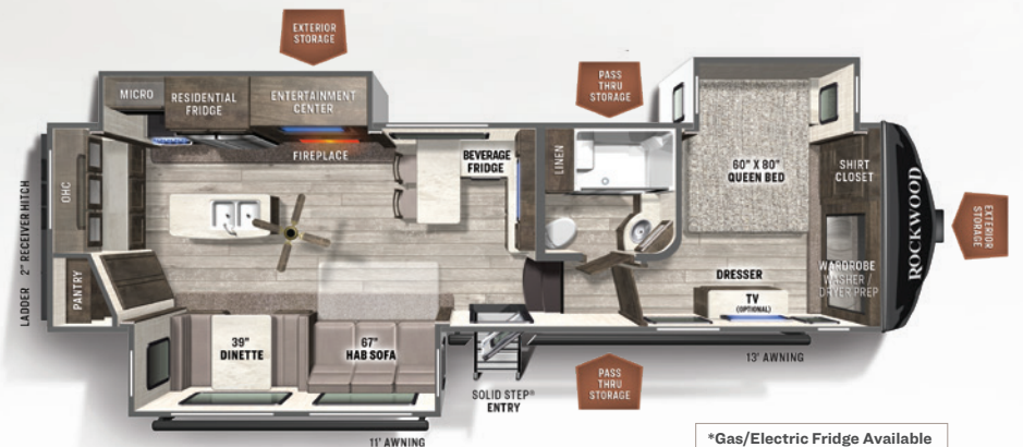
2899KS REAR KITCHEN / BAR ULTRA LITE U/VW: 10255 HITCH: 1699 AXLE: 8497 CCC: 1844 LENGTH: 36' 6" WIDTH: 8' HEIGHT: 13' 2" FRESH: 54 gal GRAY: 80 gal BLACK: 50 gal
