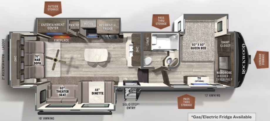
2893BS REAR LIVING ULTRA LITE U/VW: 10434 HITCH: 1675 AXLE: 8700 CCC: 1641 LENGTH: 36' 6" WIDTH: 8' HEIGHT: 13' 2" FRESH: 54 gal GRAY: 90 gal BLACK: 50 gal
