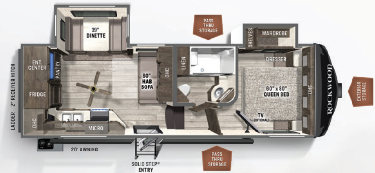
2445WS REAR KITCHEN ULTRA LITE UVW: 7764 HITCH: 1215 AXLE: 6490 CCC: 2051 LENGTH: 28' 11" WIDTH: 8' HEIGHT: 13' 1" FRESH: 54 gal GRAY: 80 gal BLACK: 40 gal
