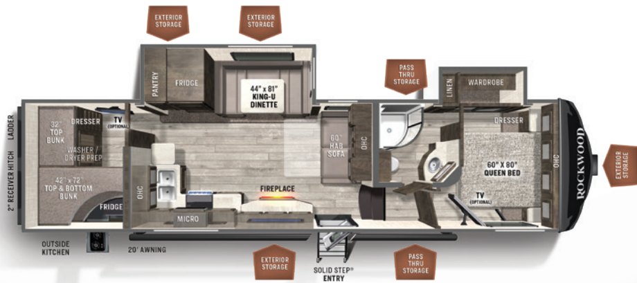
2891BH BUNKHOUSE ULTRA LITE U/VW: 9270 HITCH: 1483 AXLE: 7728 CCC: 2213 LENGTH: 36' 6" WIDTH: 8' HEIGHT: 13' 2" FRESH: 54 gal GRAY: 80 gal BLACK: 40 gal
