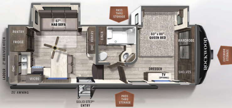
2442BS REAR KITCHEN ULTRA LITE UVW: 7950 HITCH: 1252 AXLE: 6639 CCC: 1902 LENGTH: 28' 11" WIDTH: 8' HEIGHT: 13' 1" FRESH: 54 gal GRAY: 80 gal BLACK: 40 gal
