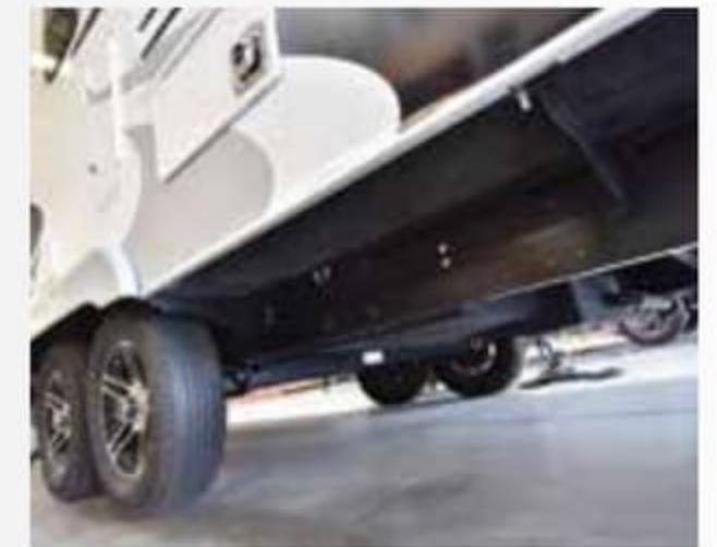
Standard HSLA e-coated frame protected against the mud, dirt and elements.
