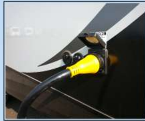
50 Amp Service w/Pre-Wire for Bedroom A/C
