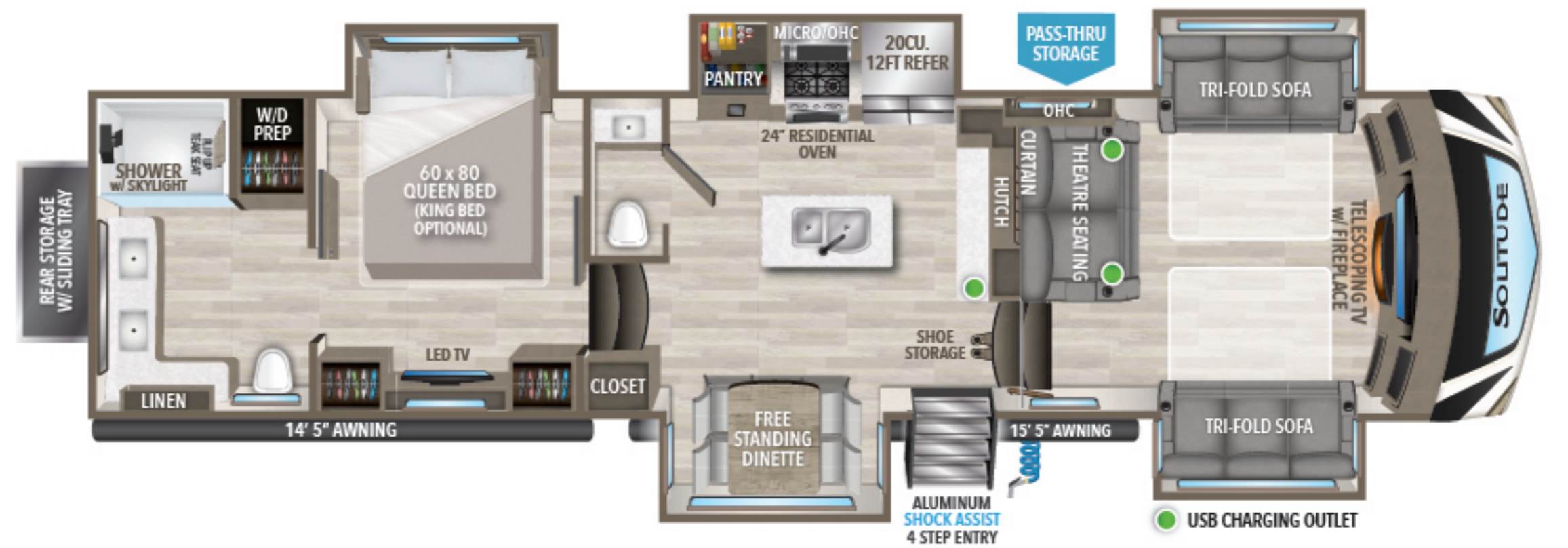
380FL UVW † 14,866 HITCH ‡ 3,052 GVWR 16,800 LENGTH † 41' 5" HEIGHT 13' 5" CAPACITY 81 106 106
