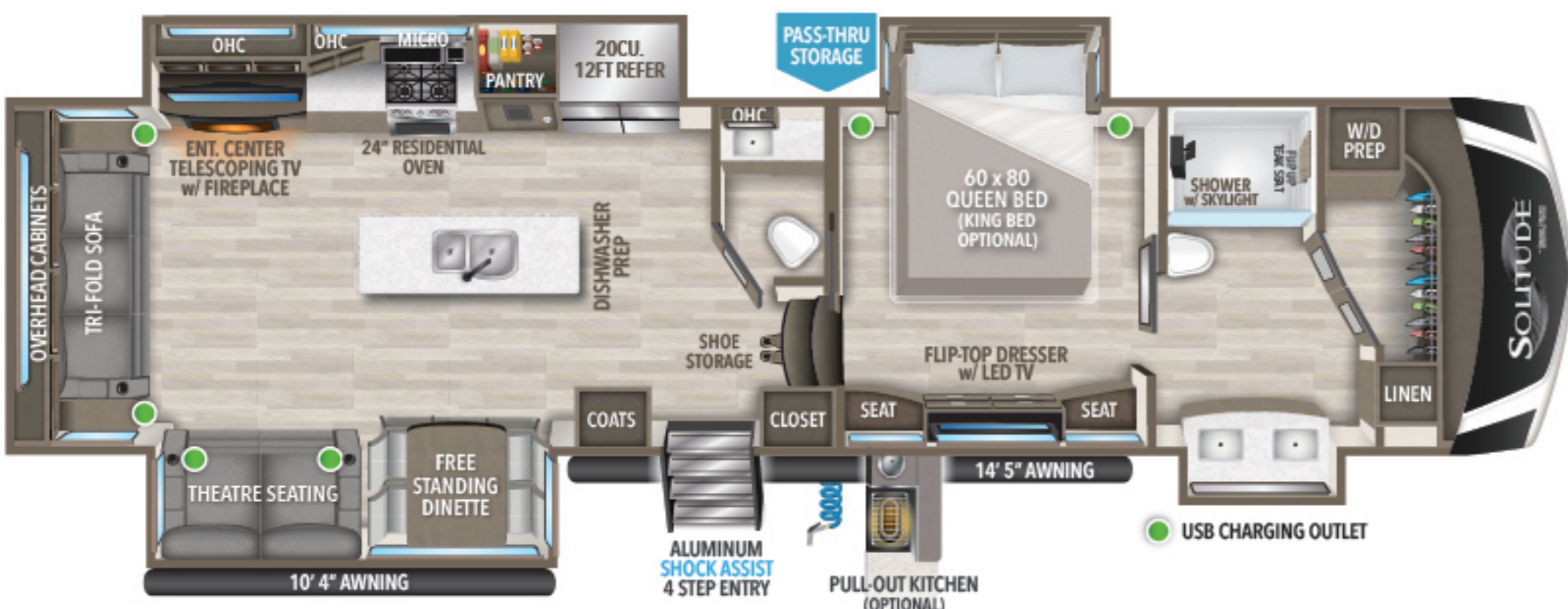
373FB UVW † 13,950 HITCH ‡ 2,800 GVWR 16,800 LENGTH † 41' 4" HEIGHT 13' 5" CAPACITY 81 106 106
